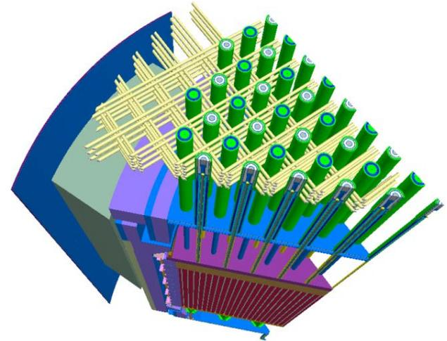
3D ray trace display of a reactor with upper concrete removed.
